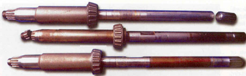
Above —Drive shafts from MerCruiser Alpha drives. The shaft at the top is broken at the O-ring groove at the upper splines. The middle shaft's lower-end splines are broken off. The bottom shaft is the most recent model, the MerCruiser Alpha Gen II. The lower-end splines have been reinforced significantly, and there is no O-ring groove machined at the upper splines. Right —A detail of the failed lower spline. Here is a good example of a ductile material that failed in pure torsion. The fracture is perpendicular to the axis of the shaft, and the surface is smooth.
