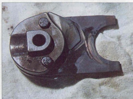
The shift plate on a MerCruiser Bravo drive. The plate is subject to wear, as shown here.
