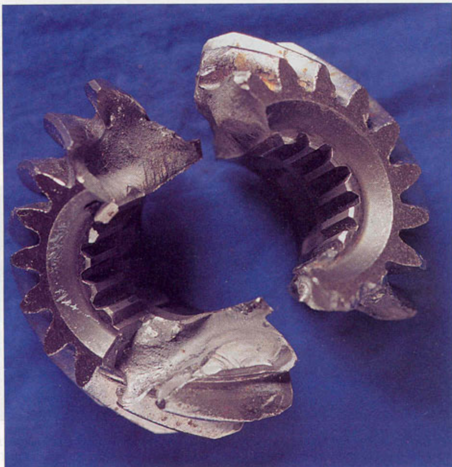
The split pinion gear pictured here is from an outdrive that struck an object, and was rebuilt without the gear's being replaced. The impact had caused a hairline crack in the gear at the root of one of the teeth. The crack started the fatigue process, which ended in the gear's failure a year later.
