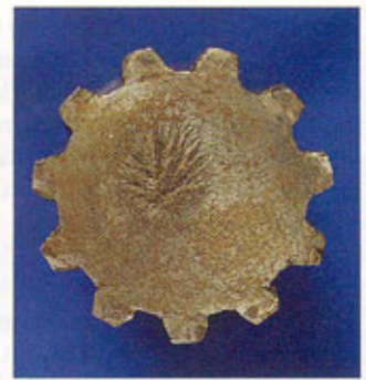
Above —Drive shafts from MerCruiser Alpha drives. The shaft at the top is broken at the O-ring groove at the upper splines. The middle shaft's lower-end splines are broken off. The bottom shaft is the most recent model, the MerCruiser Alpha Gen II. The lower-end splines have been reinforced significantly, and there is no O-ring groove machined at the upper splines. Right —A detail of the failed lower spline. Here is a good example of a ductile material that failed in pure torsion. The fracture is perpendicular to the axis of the shaft, and the surface is smooth.
