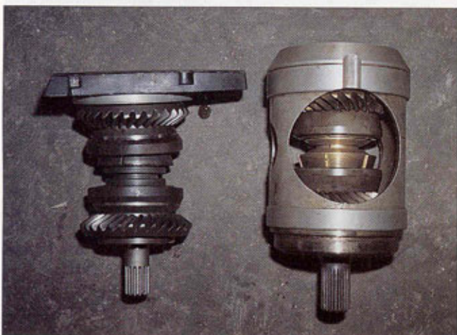
Top photos, left to right —The lower-unit drive assembly showing the pinion gear on the vertical drive shaft mated to the forward gear (left) and reverse gear (right), with the clutch dog between the forward and reverse gears; the same parts disassembled. The second photo shows that the unit shifts by sliding the clutch dog along the horizontal prop shaft so that it engages either the forward or reverse gear. The teeth on the clutch dog are not subject to impact damage, but will wear from shifting. Above, left —A MerCruiser Bravo cone clutch (left) and an OMC assembly (right). The cone works on friction, and so is prone to wear. Above, right —Detail of lower-unit gears on a MerCruiser Bravo drive. The teeth are straight cut and the gears are forged, making them particularly rugged.
