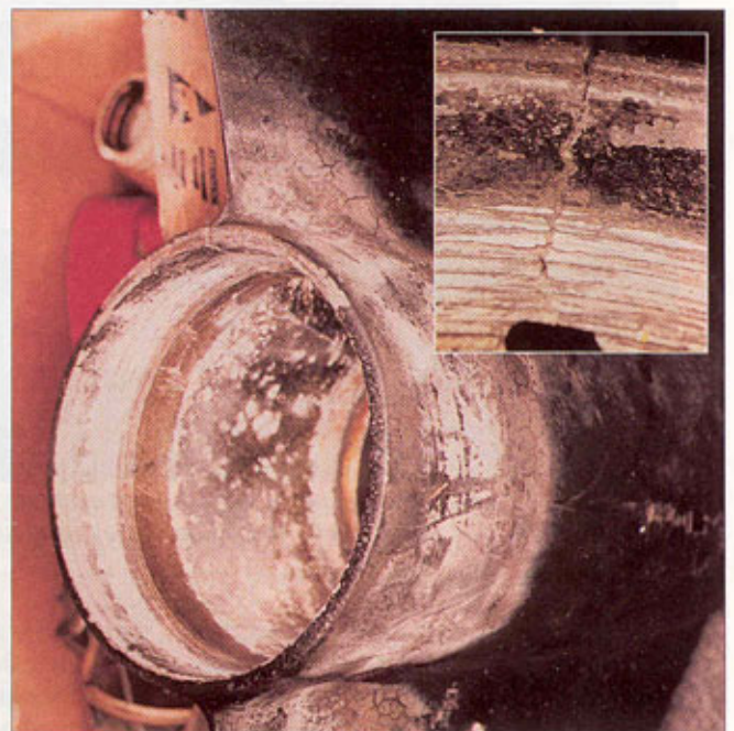
A MerCruiser lower-unit case with a crack at the top, near the web. First, the inset photo shows that debris has had time to collect in the crack. Second, the crack opens up on the outside of the case. It's most likely that the outdrive was left on during winter storage; the case filled with water and froze, and then cracked when the ice expanded.
