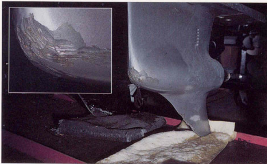
This Volvo lower unit took a direct hit to the nose of the case. The inset photo shows oil weeping out of the case through a crack caused by the impact. The case is probably beyond repair.
