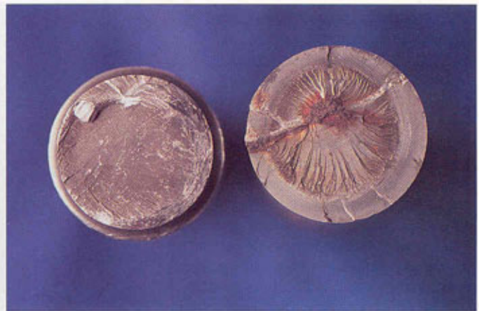
Left —Failed upper drive shafts on an older OMC stringer drive. Right —End view of the failed shafts. The same parts failed due to the same weak links. The fracture surfaces of both shafts show signs of long-term fatigue.
